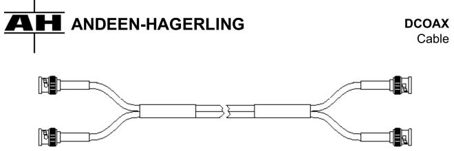
Dual, Low Noise, Coaxial Cable Optimized For Three-Terminal Capacitance Measurements
