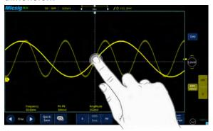
Gently double tap to zoom in, use the ruler slider to easily adjust the time base very quickly.
