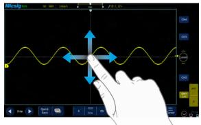
Slide your finger across the screen to quickly and precisely move the waveform along any dimension.
