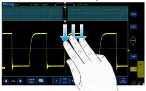
Swipe downward with three fingers simultaneously to directly access the ZOOM function directly.
