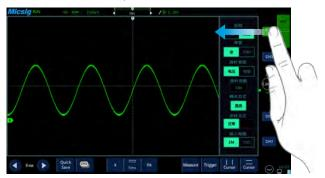
Touching and sliding the input channel buttons will open the channel's setting menu.
