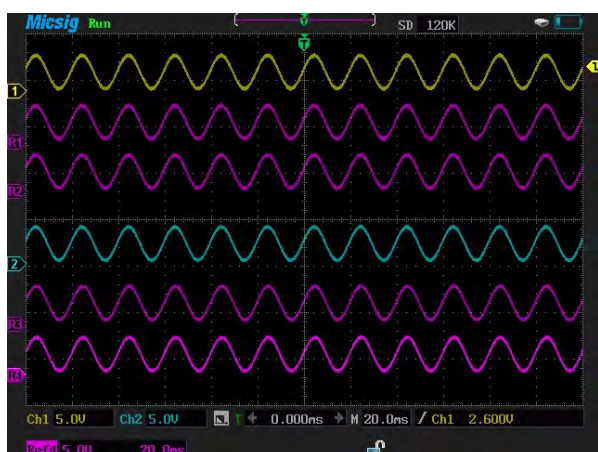
Users can choose 4 reference waveforms for comparison and analyze
