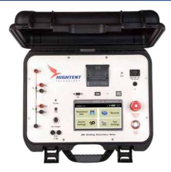
Resistance Measurement 0.1  $\mu\Omega$  - 100,000  $\Omega$
