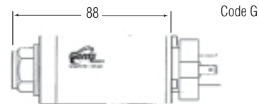
Fixed Plug to DIN 43650 Mating Connector Supplied
