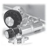
Weinschel's 940 series uses a card resistor on a disk with a movable coaxial contact (shown below) similar in nature to a potentiometer and provides an incremental range of 114 dB incremental range at 2 GHz and 60 dB at 4 GHz. Because the shunt film is connected to ground permanently, in order to achieve the extended attenuation range, the minimum loss of this type attenuator is higher (4 to 6 dB).
